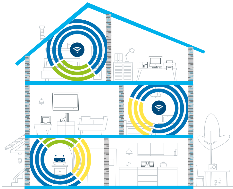
Fig. 3: The effect of bricks and concrete on a WiFi-only home network solution
